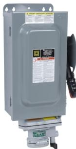
Safety switch, heavy duty, fusible, 60A, 600VAC/DC, 3 poles, 50HP, NEMA 12K, Appleton Powertite receptacle
