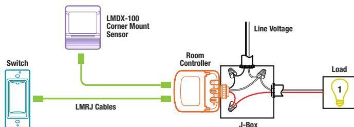
Plug DLM local network components together in any configuration using Cat 5e cables with RJ45 connectors.
