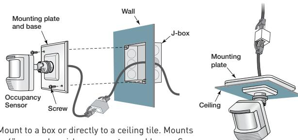
Mount to a box or directly to a ceiling tile. Mounts to 4" square box, j-boxes or octagonal boxes. See installation instructions for more details.
