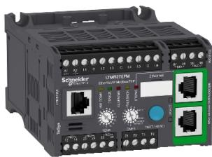
Motor controller, TeSys T, Motor Management, Ethernet/IP, Modbus/TCP, 6 inputs, 3 outputs, 1.35 to 27A, 100 to 240VAC
