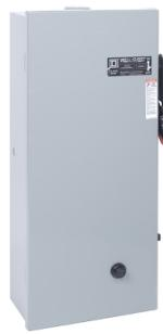
Pump Panel, NEMA Type S, Well Guard, Size 2, 45A, 5kA SSCR, 25HP, 60A Class H and K fuse clip, Motor Logic SSOLR, 110/120VAC 50/60Hz coil, NEMA 3R
