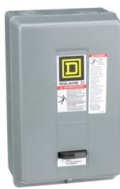
NEMA motor starter, Type S, nonreversing, Size 2, 45A, 25HP at 460VAC, 5kA SCCR, 3 phase, 3 pole, melting alloy, 120VAC coil, NEMA 1 [TAA]
