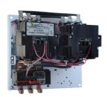
NEMA starter, Type S, reversing, horizontal, Size 3, 90A, 50HP at 575VAC, up to 100kA SCCR, 3 phase, 3 pole, Motor Logic SSOLR, 120VAC coil, open [TAA]
