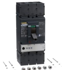
Circuit breaker, PowerPact L, 600A, 3 pole, 600VAC, 25kA, lugs, MicroLogic 3.3, 80%
