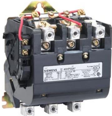
Non-reversing contactor, Size 3 1/2, Three phase full voltage, Contactor amp rating 115A, 3 wire (NO aux included), 110-120/220-240VAC 60Hz coil, Non-combination type, Enclosure NEMA type (open), No enclosure
