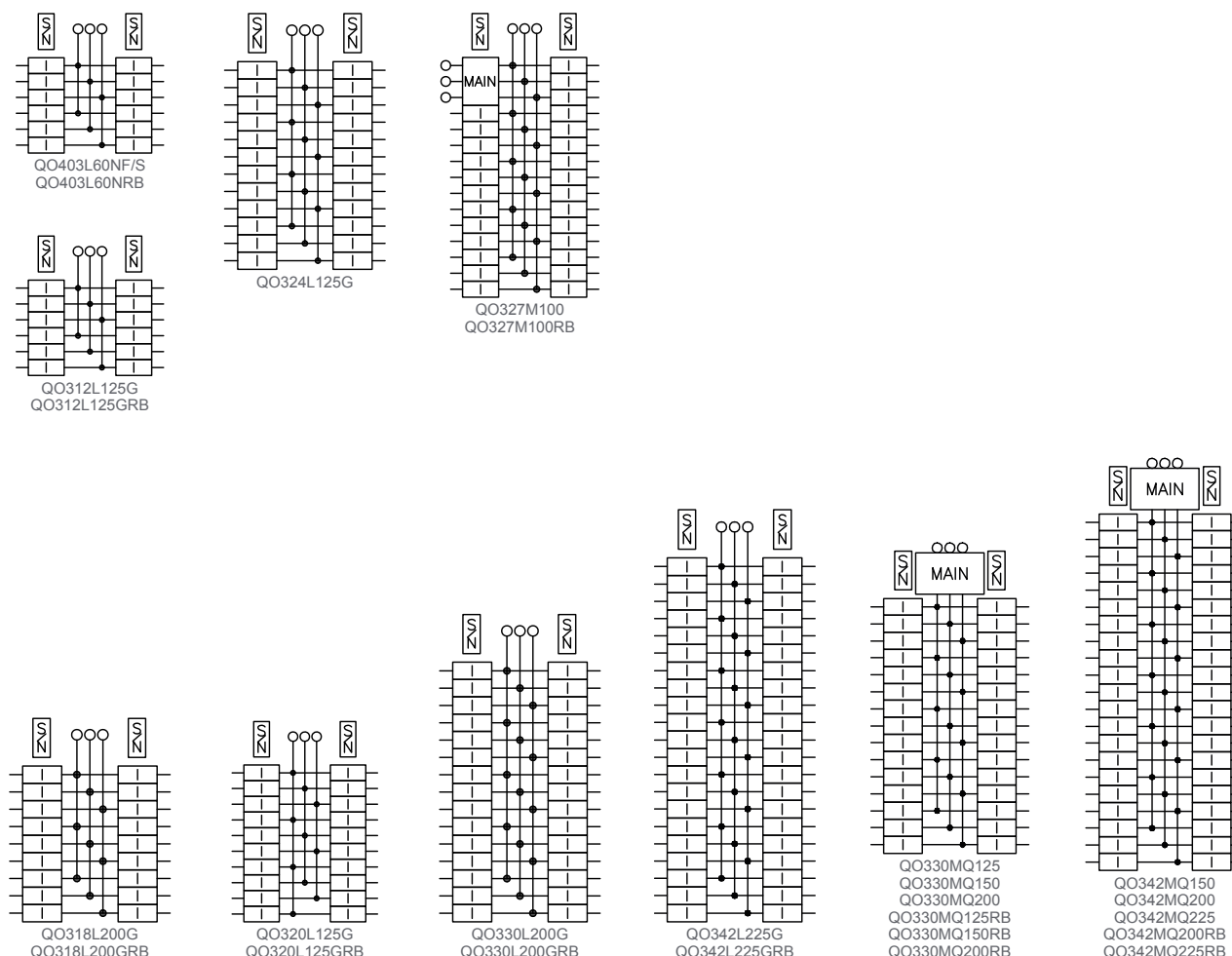
Figure 6 - QO Load Centers 3Ø – Main Lugs & Main Circuit Breaker
