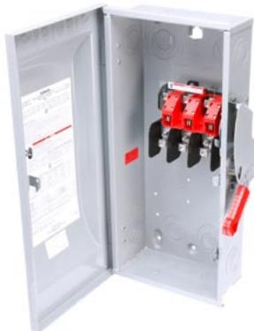
Siemens Low Voltage Circuit Protection Heavy Duty Safety Switch. 3-Pole Non-Fused in a type 1 enclosure (indoor). Rated 600VAC (100A).
