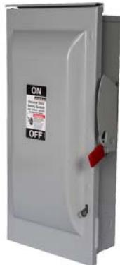
Siemens Low Voltage Circuit Protection General Duty Safety Switch. 2-Pole or 3-Pole Non-Fused in a type 3R enclosure (outdoor). Rated 240VAC (100A). Horse power: 1-PH 2-W (15), 3-PH 3-W (30), 250VDC (20). Special features: service entrance labeled suitable for 3-PH motor loads.
