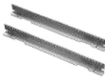
Rack Angles allow for mounting 19-in. rack equipment in 600-mm wide enclosures. Plated 14 gauge steel with .281-in. (7-mm) diameter holes (through-hole type). Twenty M5 screws and 20 clip nuts included for mounting rack angles to enclosure and for mounting equipment to rack angles.
