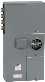
Branch unit, EZ Meter-Pak, 400A, 1 x 7 jaw socket, 208Y/120VAC, lever bypass, ringless, 1200A Cu busbar
