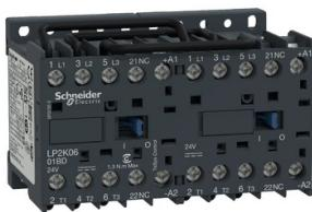
reversing Contactor, TeSys K, 3P, AC-3/AC-3e, 440V 6A, 1NC, 24V DC coil, screw clamp terminals
