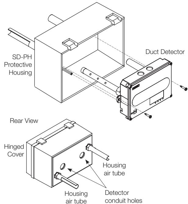
The SD-PH is easy to install and service. The hinged and transparent cover provides ready access to the detector, while keeping its status indicators visible at all times.
