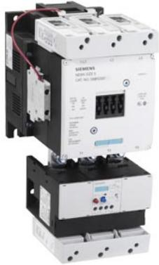
Non-reversing motor starter Size 6 Three phase full voltage Solid-state overload relay OLRelay amp range 160-630A 110-127V 50-60HZ/DC coil Combination type No enclosure
