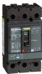
Circuit breaker, PowerPact J, 150A, 3 pole, 600VAC, 14kA, lugs, thermal magnetic, 80%
