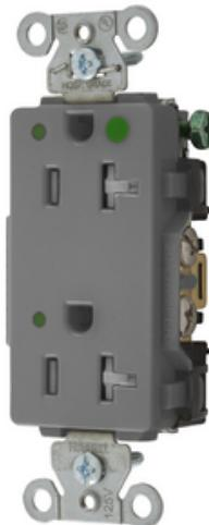
Straight Blade Devices, Tamper Resistant Decorator Duplex Receptacle, Hospital Grade, Hubbell-Pro, LED Indicator, 20A 125V, 2-Pole 3-Wire Grounding, 5-20R, Gray
