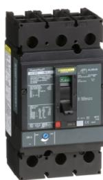
Circuit breaker, PowerPact J, 200A, 3 pole, 600VAC, 25kA, lugs, thermal magnetic, 80%
