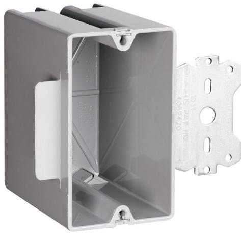
Single-Gang, Deep Bracket Box for Wood and Steel Studs with Quick/Click Entries. 3/8-inch offset for wood and steel stud mounting. For use with 3/8-inch to 5/8-inch wallboard. 100 pack.
