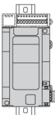
**NOTE:** Expansion modules must be mounted above the logic controller.
