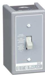
Manual Starter, fractional horsepower, 16A, 1 pole, 1 HP at 277 VAC, toggle operated, no indicator, NEMA 1 enclosure
