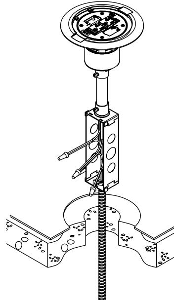
**Step 8.** Connect Poke-Thru conductors according to required device configuration. See schematic below.
