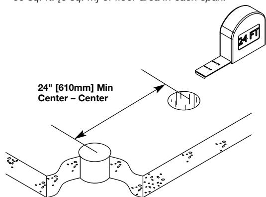
**NOTE:** Be certain to drill hole at least 4" [102mm] from any wall or pillar to leave enough room for Poke-Thru cover assembly.
