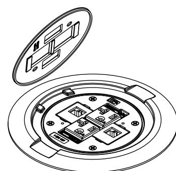
**CAUTION:** Gasket must be set in place to provide scrub water seal.
