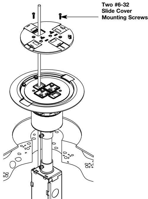
**CAUTION:** Do not over tighten cover mounting screws.
