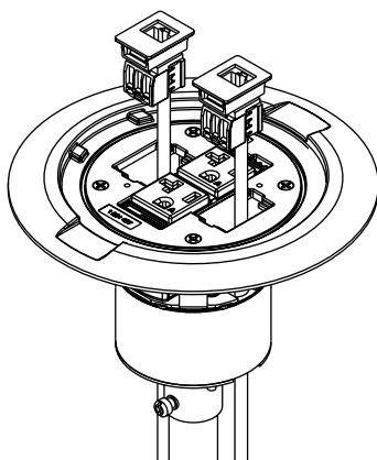
**Step 13.** Align gasket over receptacle and press bead into flange channel.
