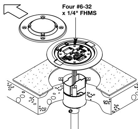
**CAUTION:** Poke-Thru cannot be rotated in hole after insertion into floor.
