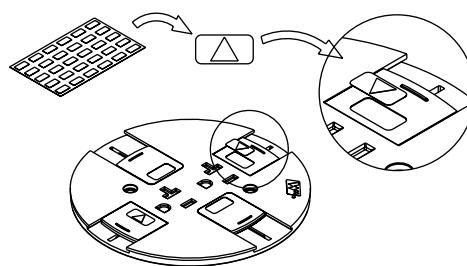
**NOTE:** The orange triangle shall only be placed on devices that are wired for isolated ground. See NEC 250-146(d).
