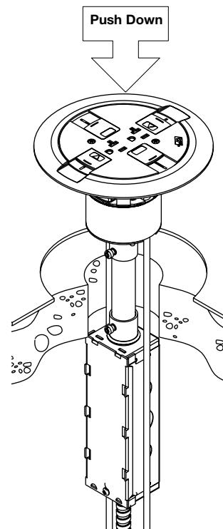
**CAUTION:** Poke-Thru cannot be rotated in hole after insertion into floor.
