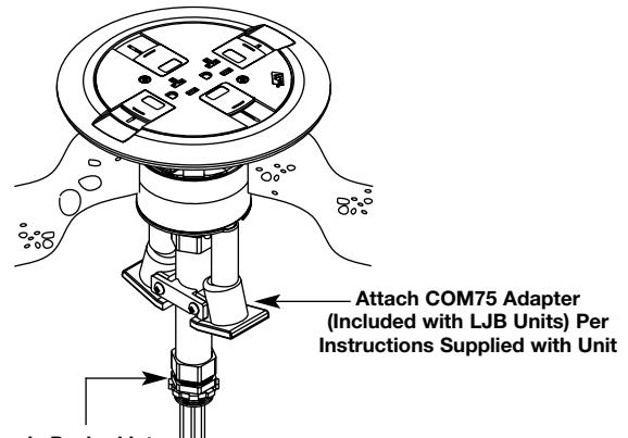
Once Poke-Thru is Pushed into the Cored Hole, from Below, Install a EMT Compression Fitting (Not Supplied) and Junction Box (Not Supplied) to the Conduit System. Complete Installation Per NEC and Local Codes.
