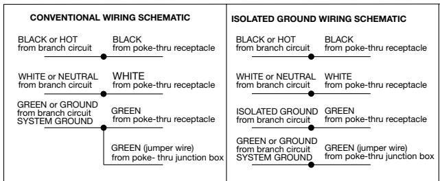
**WARNING:** Ground wire from junction box must be connected to SYSTEM GROUND.
