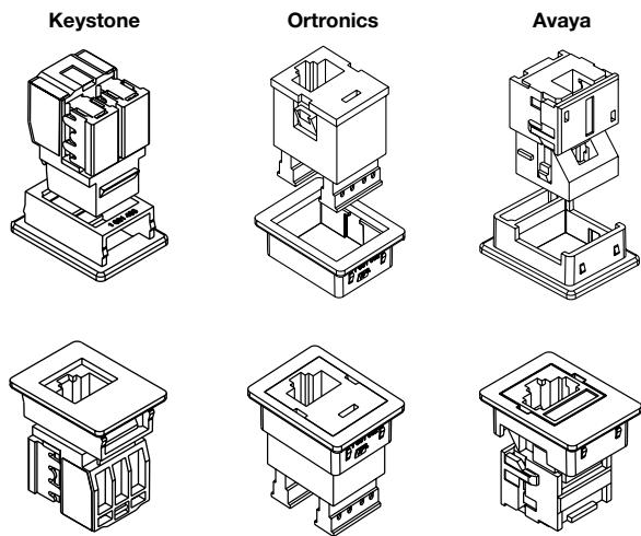
**Step 11.** For cable pass-through or empty communication port, install foam block in keystone adapter. Pass cable through adapter adjacent to foam plug. Close off non-utilized Ortronics® adapters with plastic TracJack® blank.
