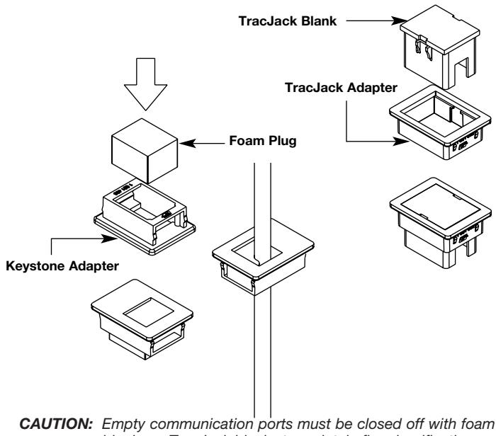
**NOTE:** To maintain UL Fire Classification, all communication modules or blank inserts (factory or customer supplied) must be UL Listed communication circuit accessories, and must fit securely in the supplied communication brackets with no visible openings between the module and bracket. Supplied foam plugs must be used when passing cables through the communication openings.
