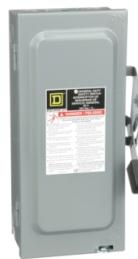
Safety switch, general duty, fusible, 3 pole, 4 wire, 240VAC, 60A, Type 1, with neutral
