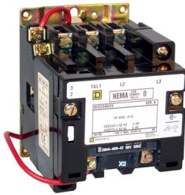
NEMA Contactor, Type S, nonreversing, Size 0, 18A, 5HP at 575VAC, 3 phase, up to 100kA, 3 pole, 208VAC coil, open [TAA]
