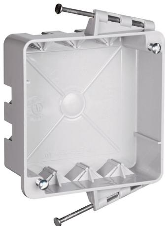
4-inch Square Box with threaded mounting holes, captive mounting nails each end. 3 Auto/Clamps each end, 2 on side opposite to nails. Two #8Mounting Screws Factory Installed.
