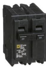
Mini circuit breaker, Homeline, 20A, 2 pole, 120/240VAC, 10kA AIR, standard type, plug in, UL
