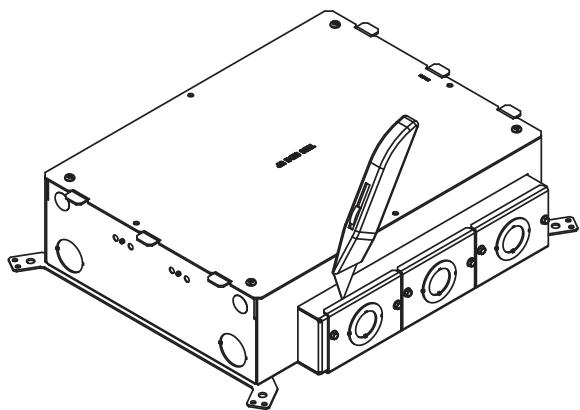
**Step 3.** Remove device plate on the inside of the floor box.
