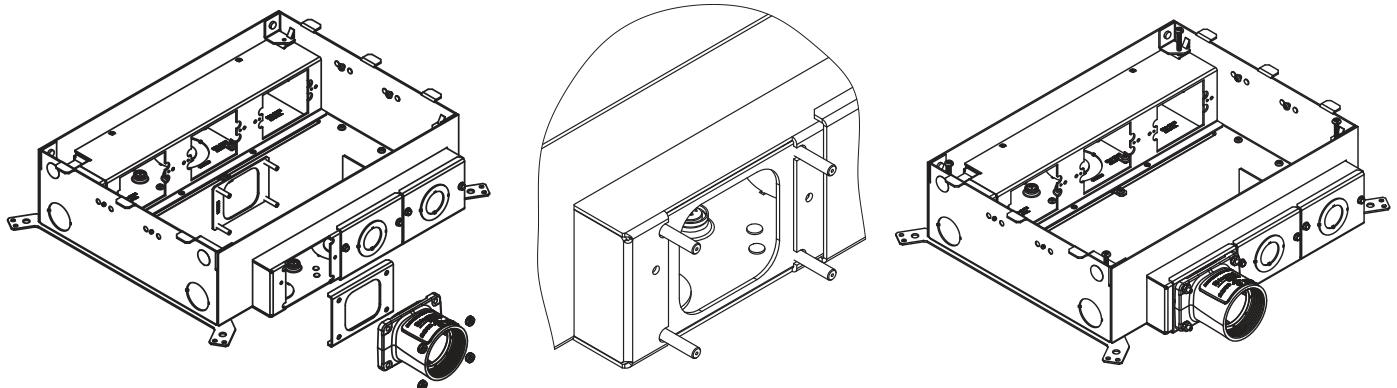
**Step 6.** Complete the installation by attaching 2 inch conduit to the Hub.
