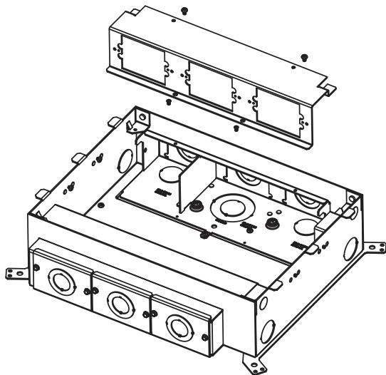
**Step 4.** Remove knock out plate by tapping the plate loose from the box as shown.
