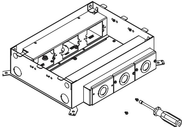
**Step 2. For On-Grade Boxes:** To facilitate the removal of the knock out plate, use a utility knife to score the paint around the edges of the plate as shown.
