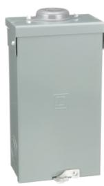
Circuit breaker enclosure, QO, 1 phase, 2 spaces, 100A, NEMA3R, UL
