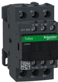
IEC contactor, TeSys Deca, nonreversing, 25A, 15HP at 480VAC, up to 100kA SCCR, 3 phase, 3 NO, 230VAC 50/60Hz coil, open
