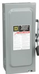
Safety switch, general duty, fusible, 2 pole, 3 wire, 240VAC, 60A, Type 1, with neutral
