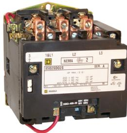
**NEMA Contactor, Type S, nonreversing, Size 2, 45A, 25 HP at 575 VAC, 3 phase, up to 100 kA, 3 pole, 480 VAC coil, open [TAA]**
