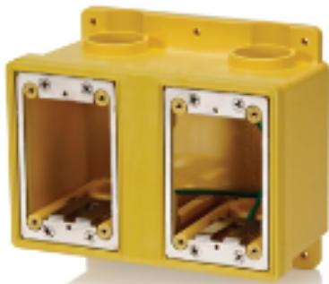
FD Box, Two-Gang, 67.3 Cubic Inch Capacity, 1" unthreaded conduit openings with reducers for 3/4" and 1/2" conduit, includes plugs for unused openings and stainless steel device mounting plates with ground wire, industrial grade - YELLOW
