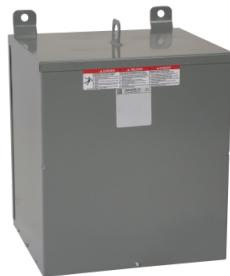
Transformer, dry type, encapsulated, 15kVA, 1 phase, 240x480V primary, 120/240V secondary, 15B, 115C rise [TAA]
