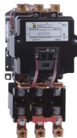
NEMA Motor Starter, Type S, nonreversing, Size 4, 135A, 100 HP at 460 VAC, 3 phase, 3 pole, melting alloy, 208 VAC coil, open, 10 kA SSCR [TAA]
