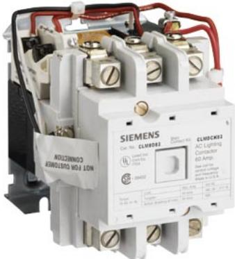
Mechanically held lighting contactor, Contactor amp rating 60A, 0 N.C. / 3 N.O. poles, 110VAC 50HZ/120VAC 60HZ coil, Non-combination type, Enclosure NEMA type (open), No enclosure
