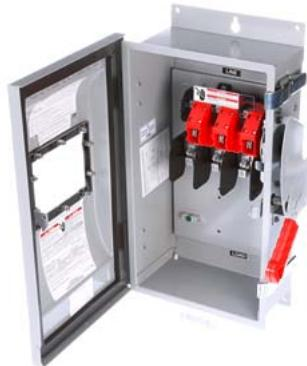
Siemens Low Voltage Circuit Protection Heavy Duty Safety Switch. 3-Pole Non-Fused in a type 12 industrial enclosure. Rated 600VAC (30A). Special features: viewing window.
