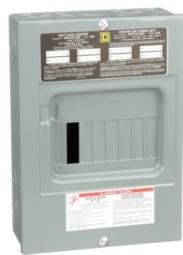
Load center, QO, 1 phase, 8 spaces, 16 circuits, 100A fixed main lugs, NEMA1, surface cover
