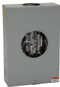
Meter socket, ringless socket, lever bypass, 200 A, 600VAC, 3 phase, 7 jaw, jaw release, OH/UG
