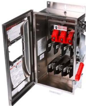
Siemens Low Voltage Circuit Protection Heavy Duty Safety Switch. 3-Pole 3-Fuse Fused in a type 4/4X 304 grade Stainless Steel enclosure. Rated 600VAC (60A). Special features: viewing window.
