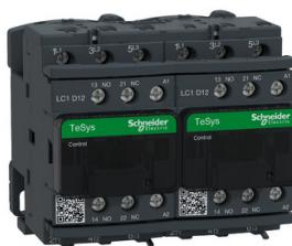
IEC contactor, TeSys Deca reversing, 12A, 7.5HP at 480VAC, 3 phase, 3 pole, 3 NO, 120VAC 50/60Hz coil, open style
