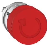
Emergency stop head, Harmony XB4, switching off, metal, red mushroom 30mm, 22mm, trigger latching turn to release
