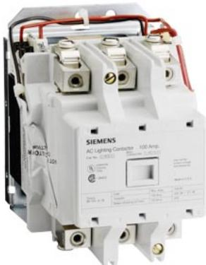
Mechanically held lighting contactor, Contactor amp rating 100A, 0 N.C. / 3 N.O. poles, 277VAC 60HZ coil, Non-combination type, Enclosure NEMA type (open), No enclosure
