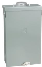
Load center, Homeline, 1 phase, 4 spaces, 8 circuits, 125A fixed main lugs, NEMA3R, gnd bar
