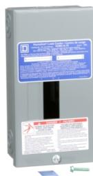
Load center, Homeline, 1 phase, 2 spaces, 4 circuits, 70A fixed main lugs, NEMA1, surface cover
