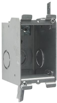
Single gang metal box. Swing bracket for mounting adjusts 11/4" down to 1/4". Four 3/4" x 11/4" KOs plus integral Romex clamp.
