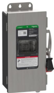
**Safety switch, heavy duty, unfused, viewing window, NEMA 4X, 600V, 30A, 3 pole, neutral installed, ground lugs**
