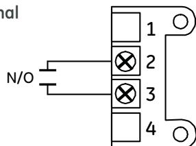
Six contact terminal block wiring
