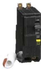
Mini circuit breaker, QO, 20A, 2 pole, 120/240VAC, 10kA, bolt on, 6mA grd fault A, pigtail [TAA]
