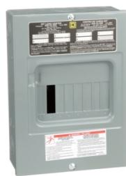
Load center, QO, 1 phase, 6 spaces, 12 circuits, 100A fixed main lugs, NEMA1, surface cover
